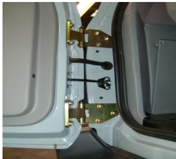
New, reinforced door hinges
